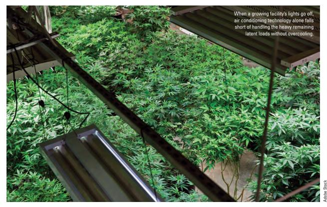
conditioning that is unable to handle the humidity loads. Generally, they're designed to fix a sensible cooling-only room's inadequacies.
