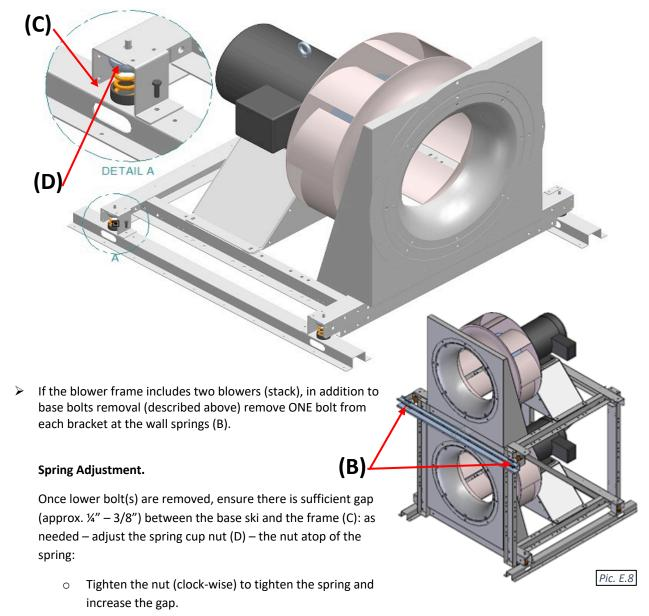
o Loosen the nut (counter-clock-wise) to loosen the spring and reduce the gap.
