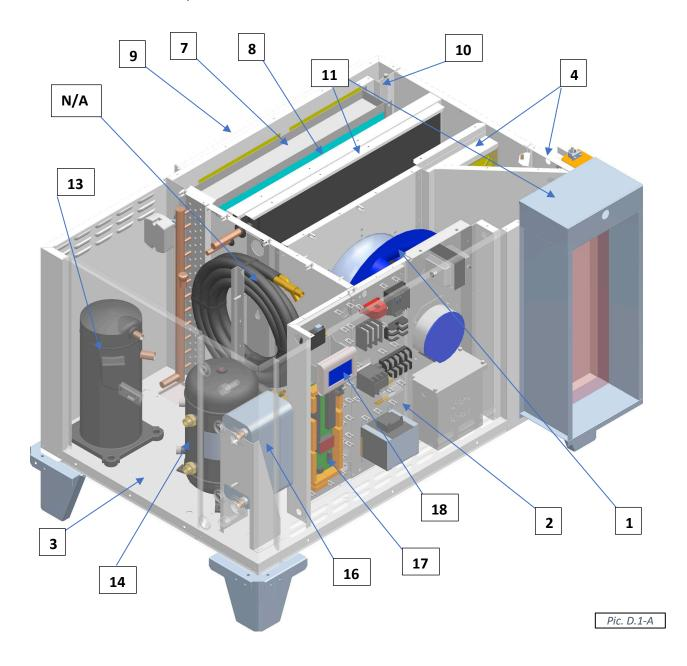
• Main Blower (1) is in the main blower compartment next to the Main Electric Panel (2) and Compressor Compartment (3).
