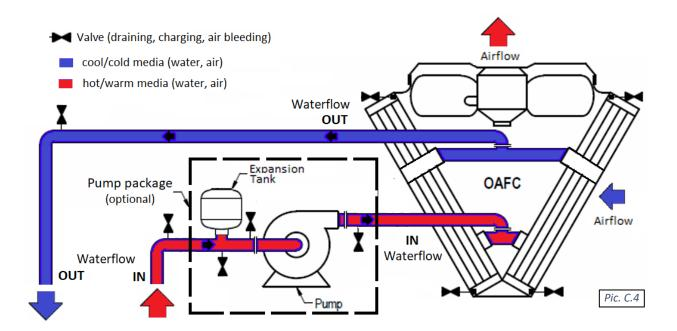
For more details on dry cooler piping connection refer to Installation Manual, submittal documentation etc. as well as local Codes and proper field practices.
